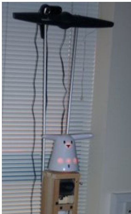
Figure 1: The Nabaztag on a pedestal (with array microphone, web-cam, and a PIR sensor)
